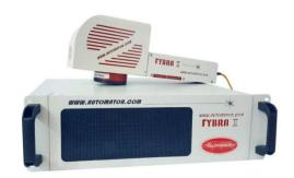
FYBRA<sup>II</sup> comes with three main components: the BOX contains the source and the electrical components, The HEAD with a galvanometer for fast x/y movement and focal lens and the FIBER optic cable that connects the two. The AUTOMATOR FYBRA<sup>II</sup> couples the stability of a fiber laser with our proprietary EuGENIUS<sup>TM</sup> software to create market leading "power-to-the-part" performance.
